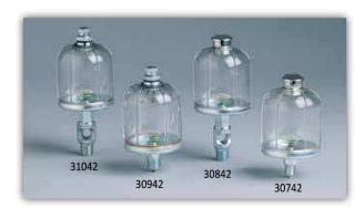
Vari-Feed wick oilers are used to provide a controlled amount of oil to a bearing or other machinery part. The principle of delivery combines gravity feed with capillary action in the wick to provide a constant feed rate of oil regardless of the fill level in the reservoir. Feed rate is determined by the viscosity of the oil and the type of wick being used.
