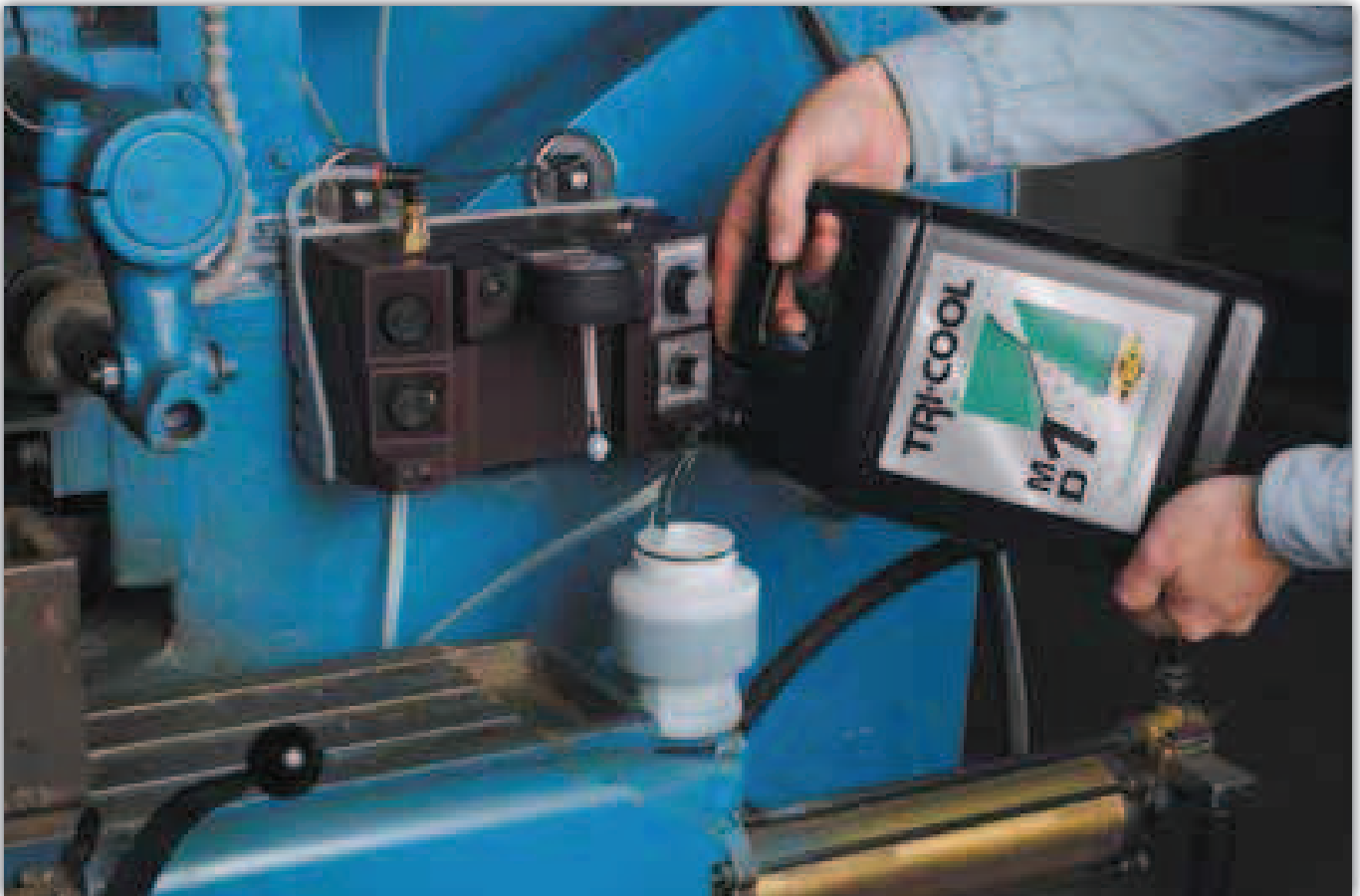
Micro-dispenser being filled with Tri-Cool MD-1 lubricant
