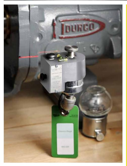
Trico gives you even more with this fool-proof method of installing the oiler – minimizing installation, reducing downtime and eliminating confusion.
